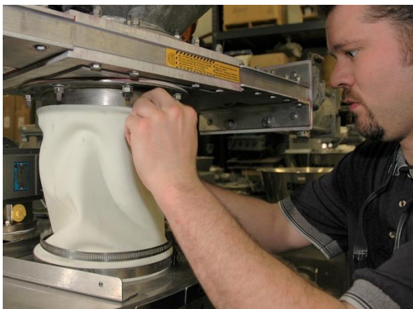
Any electrical, plumbing or other connections to the gravimetric feeder must be made with flexible conduit/piping/tubing to have minimal effect on the movement of the gravimetric scale.
