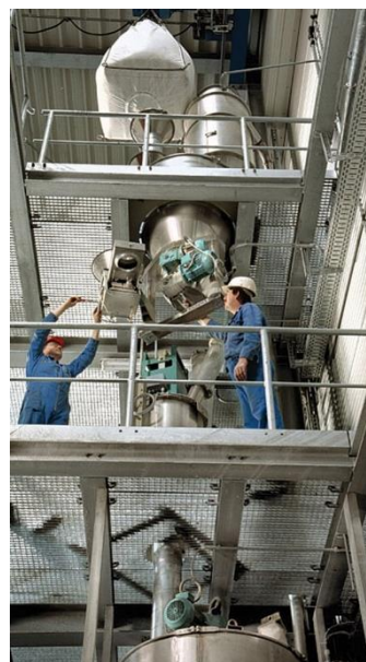
Preventive-maintenance programs are offered by some material-handling equipment suppliers. These should include a feeder audit and recommendations by a field-service engineer for improving feeder performance.
