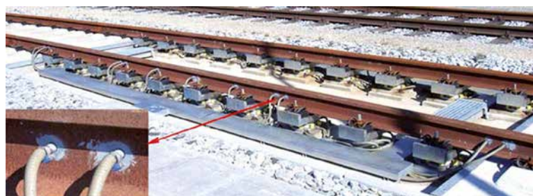
Fig. 5: View of test zone 1 and detail of shearing force sensors
