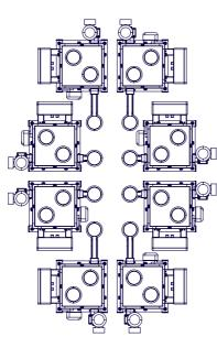
Small footprint due to asymmetric design in combination with extended discharges.
