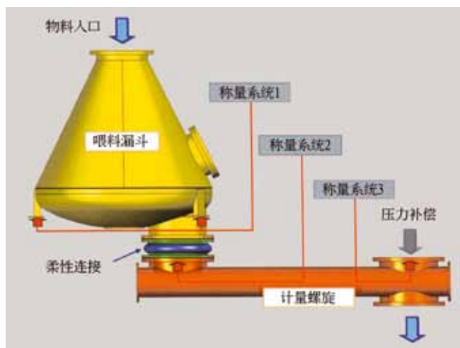
图 9: 螺旋式喂料器原理 Figure 9: Principle of a screw weighfeeder
